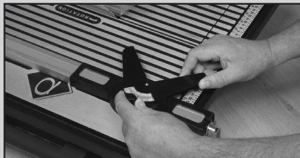
Slacken the thumb screw and set the required angle of cut.
