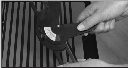
Slide the Mitre Guide into place on the Rip Guide.
